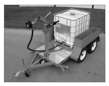
The ANSUL Master Foam nozzle is an accurate and durable self-educting foam nozzle with superior stream quality and reach. This monitor nozzle is available in your choice of 350, 500 or 750 gpm at 100 psi (1,325, 1,893 or 2,839 Lpm at 7 bar). Fog angle is user adjustable between 120° wide fog and straight stream. The nozzle baffle is easily removed for flushing debris.
